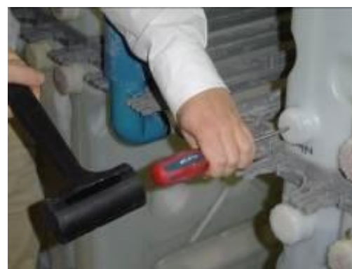
Figure 23 - Puncturing hole to drain blank module
