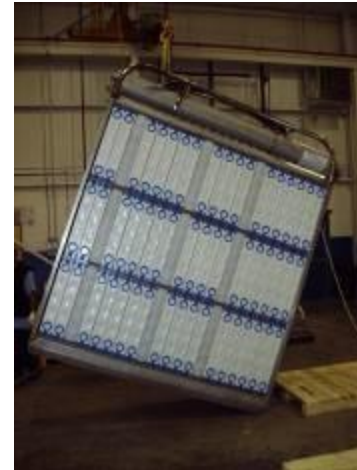
Figure 14 - Lowering cassette on a clean level surface
