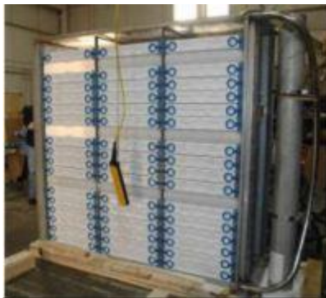
Figure 7 - Crane should be located on this side of cassette
