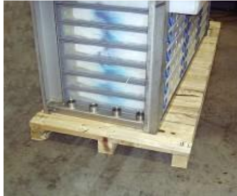
Figure 6 - Screwing the wood to cassette pallet
