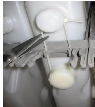
Figure 18 - Cutting the tie wrap
